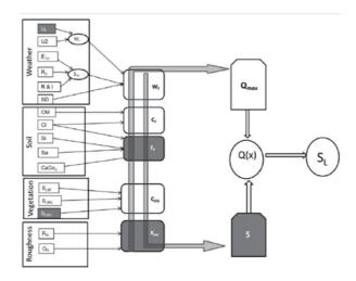
Fig. 12. Soil loss (SL) and mass transport Q(z) calculation steps in RWEQ derived by Youssef (2012)\*
