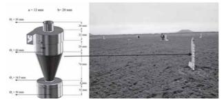
Fig. 11. BEST sediment trap (BASARAN et al., 2011)
