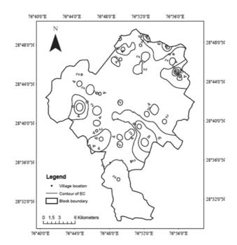
Fig. 3. Contour map of EC of groundwater in Bahadurgarh block
