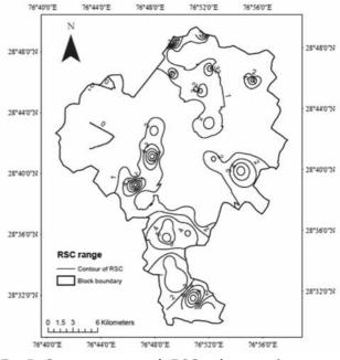
Fig. 5. Contour map of RSC of groundwater in Bahadurgarh block
