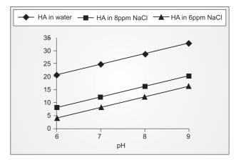
Fig. 1. Viscosity measurement HA solution in different solvents and pH
