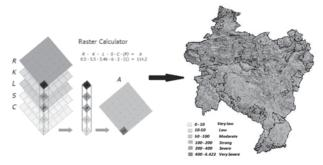
Fig. 8. Soil loss prediction process for Sakarya Basin
