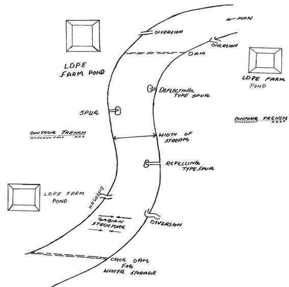
Fig. 1. Layout map of drainage line treatment of Makkowal and Takaral Watersheds
