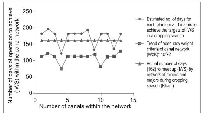
Fig. 2. Adequacy and estimated number of days required during Kharif season within canal network to achieve irrigation water supply (IWS)
