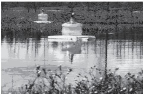
A static floating chamber measuring the rate of buildup of CO<sub>2</sub> and CH<sub>4</sub> gases over time inside the chamber
