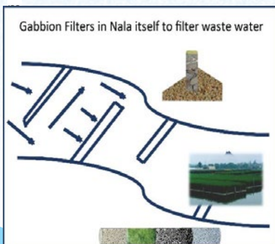
Fig. 10: Schematic view of in situ filtration system for waste water management
